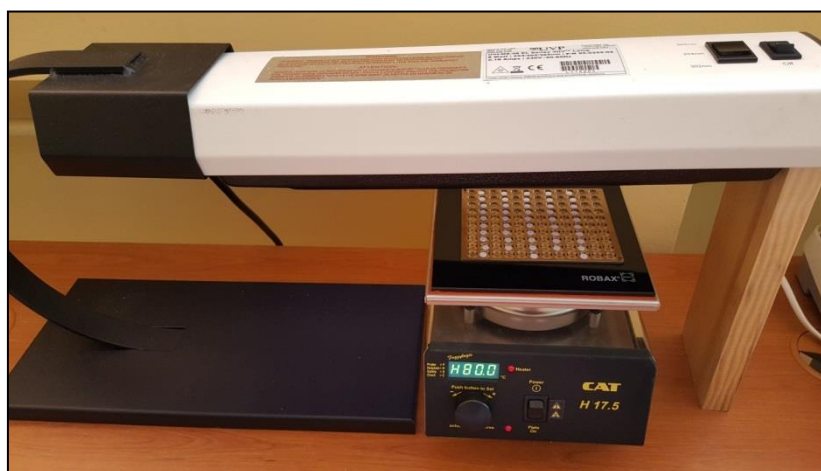
Fig. 6.7: UV LMS-38 8W lamp with HC 17.5D heating plate and TL detectors arranged on it.
